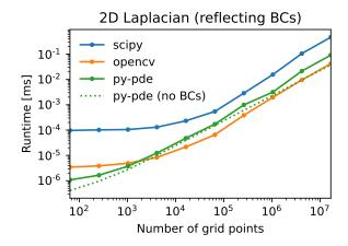
Note that the call overhead is lower in the *py-pde* package, so that the performance on small grids is particularly good. However, realistic use-cases probably need more complicated operations and it is thus always necessary to profile the respective code. This can be done using the function <code>estimate\_computation\_speed()</code> or the traditional timeit, <code>profile</code>, or even more sophisticated profilers like pyinstrument.
