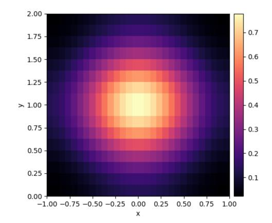
This example shows how to solve the diffusion equation on a Cartesian grid.
